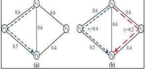
Fig: 2. Motivation for Protecting a Logical Link with Multiple Backup Paths
