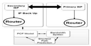
Fig: 1. Architectural Design for Selecting Backup Path
